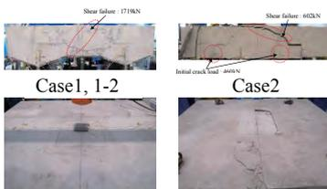
Fig. 3: Specimens for experiments
