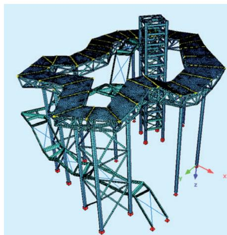
Fig.2 FEM model for check calculations
