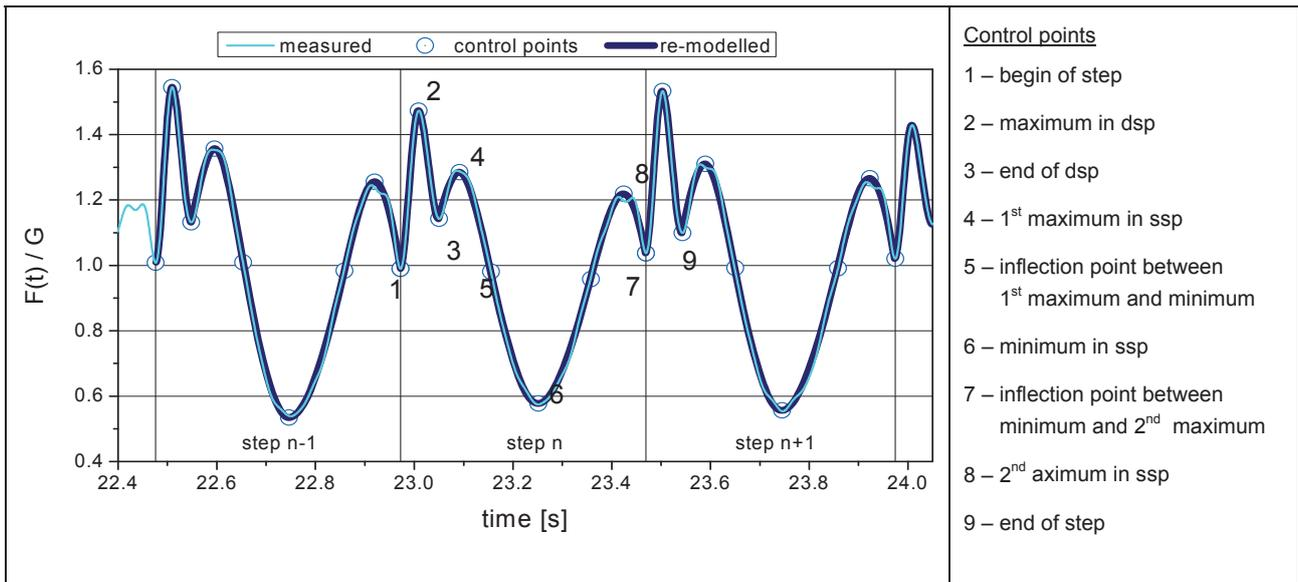
Fig. 1. Re-modelling the walking induced loads for each individual step based on characteristic points
