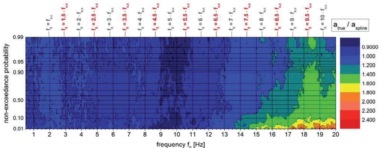
Fig. 2. Contour plot of the ratio of the true maximum acceleration to the maximum acceleration applying the re-modelled load time series, frequency distribution of the ratio for the 5%, 50% and 95% percentile
