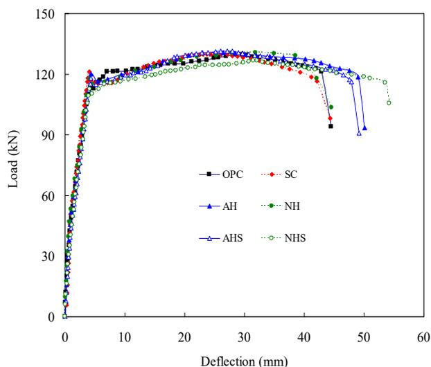
Fig. 2: Comparison of the load-deflection curves for beam specimens at the age of 28 days
