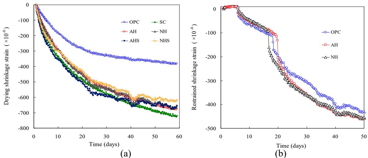
Fig. 1: Free and restrained drying shrinkage strain
